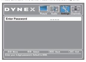
**4** Press the number buttons to enter the four-digit password. The *Parental Controls* menu opens.
